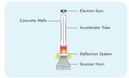
An Electron Gun is housed in a thick vessel where electrons are accelerated in an accelerator tube & directed to a scanning device magnetically to scan.
